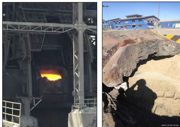
Peirce Smith Converter in operation and precast shapes after the campaign.
