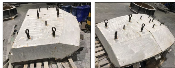
Precast shapes after drying.
