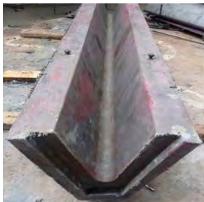
Precast Anode Launder
