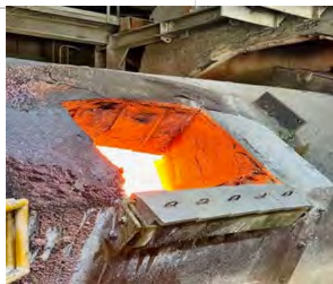
Anode Furnace Bib precast shape using ARMORMAX®
