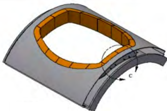
Precast shape concept for Noranda Reactor
