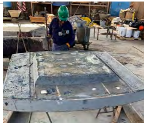
Anode Furnace Cover lined with no cement product
