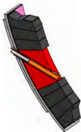
Precast Tuyere Block and Tuyere concept
