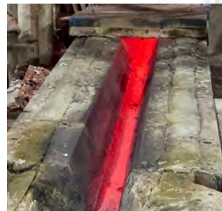
Precast inserts without sacrificial lining
