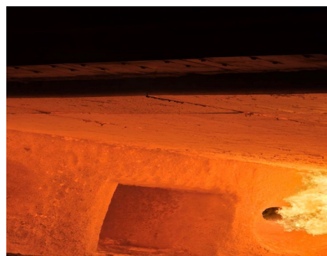
NANO-TEK® 70 and INSULMIX® 2025 during first heat-up
