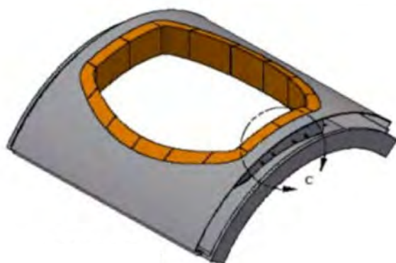
Precast shape concept for Noranda Reactor
