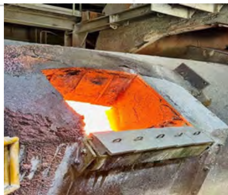
Anode Furnace Bib precast shape using ARMORMAX®
