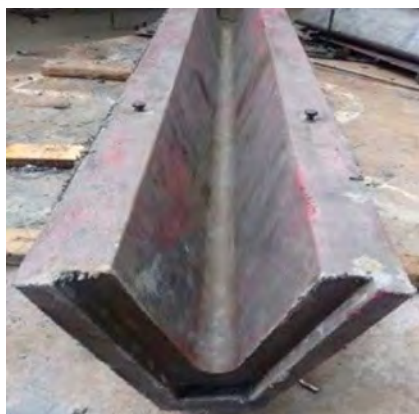
Precast Anode Launder
