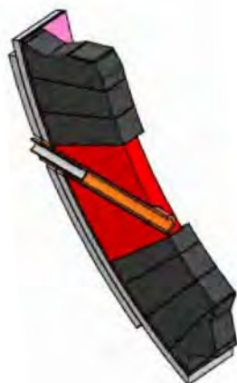
Precast Tuyere Block and Tuyere concept
