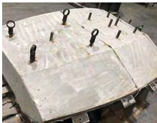
METAL-ROK® Precast Shape for Peirce-Smith Converter
