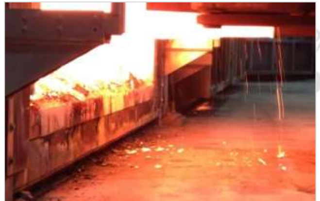
ARMORMAX® sill after 18 months in service
