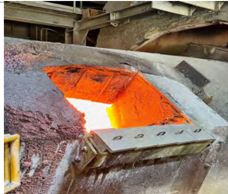
Anode Furnace Bib precast shape using ARMORMAX®
