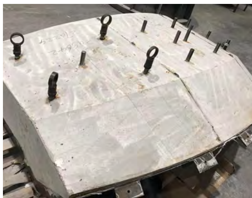
METAL-ROK® Precast Shape for Peirce-Smith Converter
