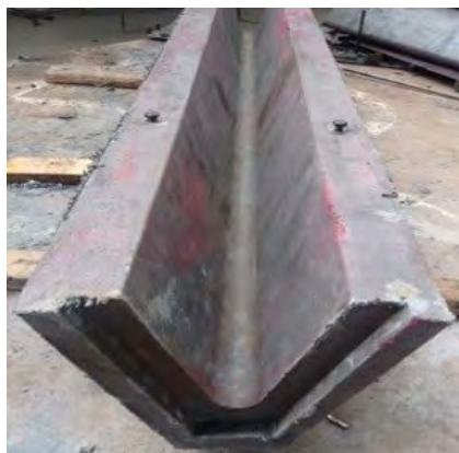
Precast Anode Launder
