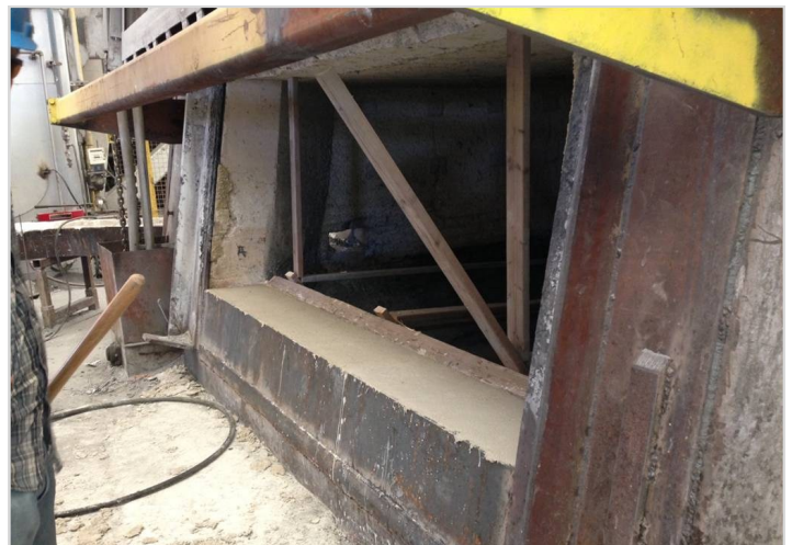
Completed reverb furnace sill with ARMORMAX® 70 AC
