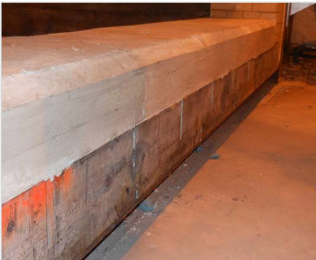
ARMORMAX® 70 SR in forge furnace sill
