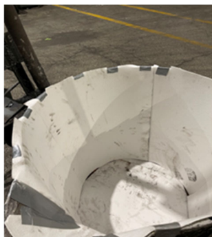
Line the ladle shell with Ceramic Paper or corrugated cardboard.
