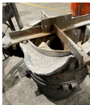
Install sidewall DRI-FIRE lining in layers using tamping and forking tools.
