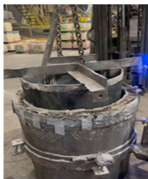
Remove ladle form once flames have subsided, and are no longer visible.
