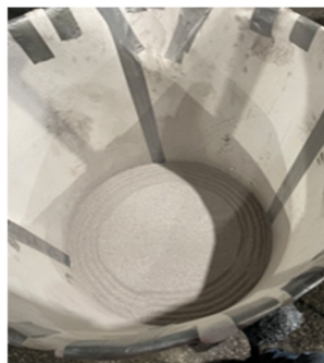
Install ladle lining bottom in layers, using tamping and forking tools.
