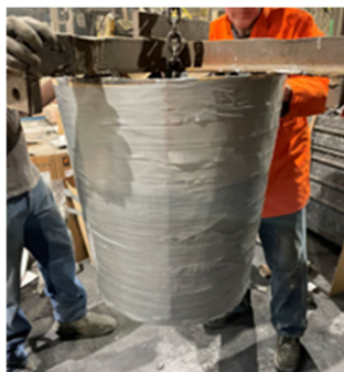
Cover form with Ceramic Paper or corrugated cardboard.
