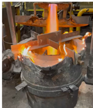
Apply heat to the ladle bottom using a torch, wood, fuel, or other heat source.
