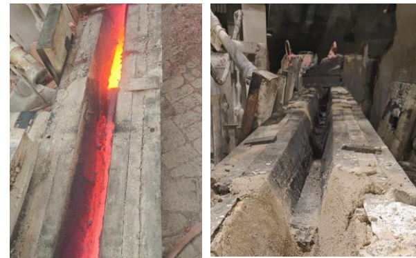
Launder condition during and after 65 heats of use
