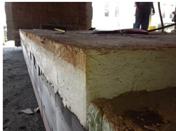
Heat treat furnace car deck perimeter after 5 months in service
