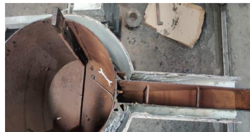
Make a form and groove arrangement for slag stone to make a T-Spout ladle.
