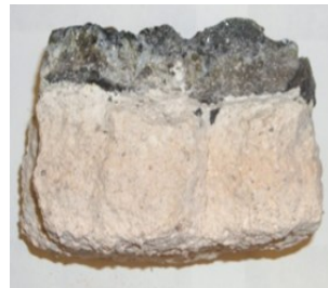
Slag and metal infiltration of conventional silica-based dry vibratable
