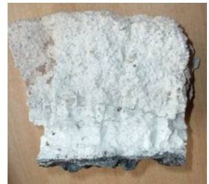
Slag and metal infiltration of LGS silica
