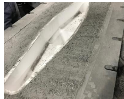
CeraLoop™ installed with DRI-VIBE® back-up
