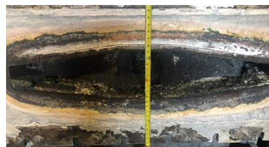
First CeraLoop™ after inductor removal, remained intact during productions
