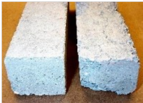
TUFFLOOR® vs Standard Concrete Thermal Cycling to 1400°F (760°C)
