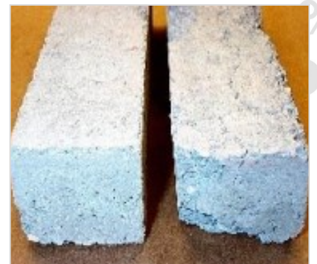
TUFFLOOR® vs Standard Concrete Thermal Cycling to 760°C (1400°F)
