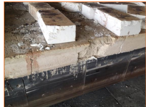
Closeup of ARMORMAX 70 SR after 5 months
