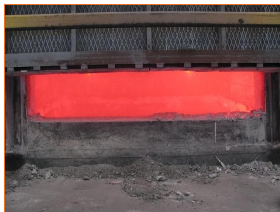
ARMORMAX® 70 AC sill after 10 months service
