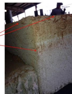
Notice that the Armormax 70 SR hasn't lost a top or corner edge after 5 months of service. The edges are as sharp as the day we cast them.
