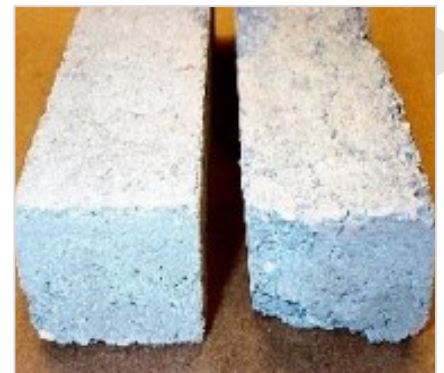
TUFFLOOR® vs Standard Concrete Thermal Cycling to 760°C (1400°F)
