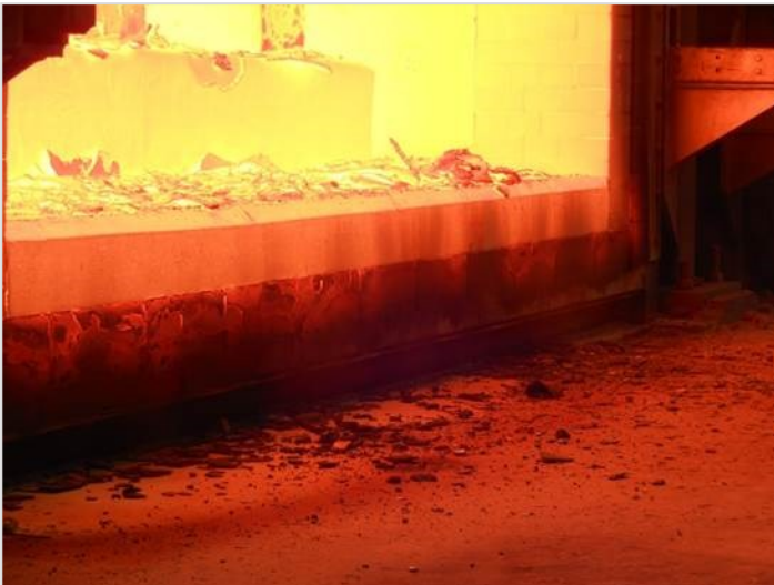
ARMORMAX® sill after 1 month in service
